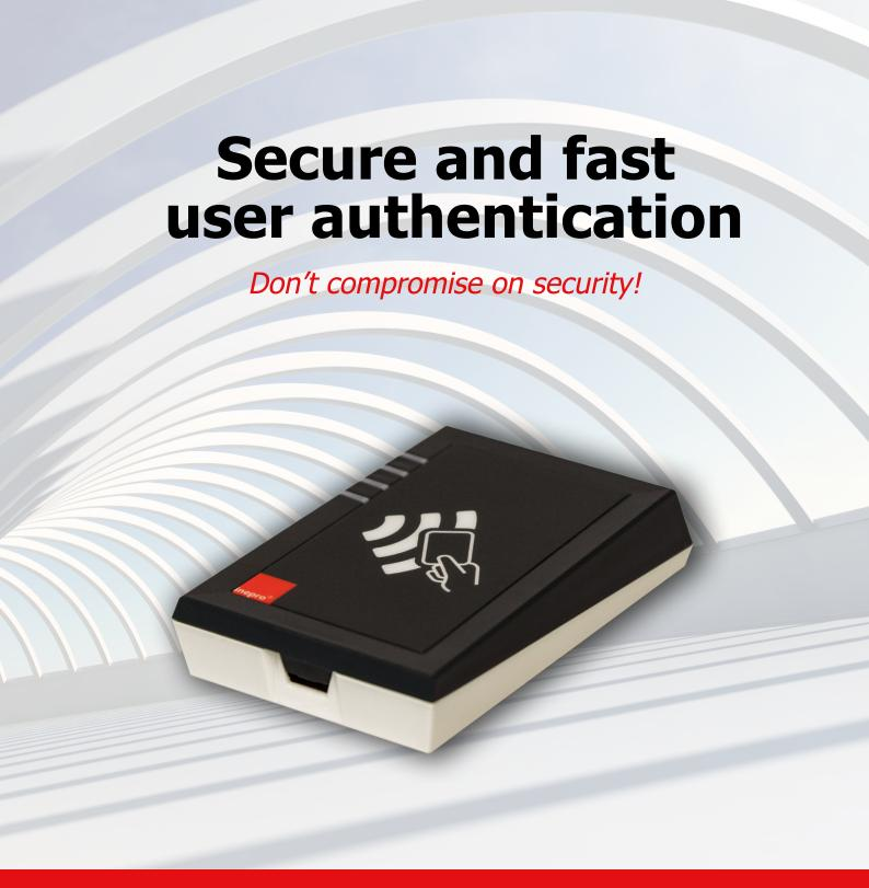
Inepro's SCR708.I is a contactless/RFID reader that can be built into different devices such as a Multi Functional Printer, cash register, laptop or pc. The USB-version is easy to configure and communicates via keyboard emulation.
